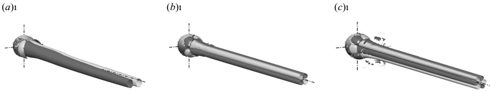
FIGURE 6. Three types of steady flow. Isosurfaces of axial vorticity at Pr = 0.72 . (a) Regime I: bifid wake with symmetry plane at Ri = 0.2 and Re = 400 ; \omega_x = \pm 0.1 . (b) Regime II: wake with four vorticity threads and two symmetry planes at Ri = 0.6 and Re = 1100 ; \omega_x = \pm 0.01 . (c) Regime III: wake with six vorticity threads and three symmetry planes at Ri = 0.7 and Re = 1300 ; \omega_x = \pm 0.001 .
